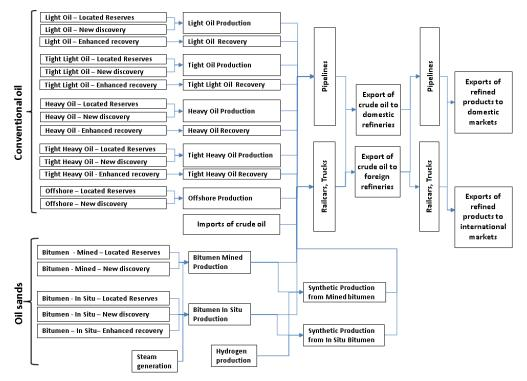
Figure 23. Schematic representation of the oil supply sector
