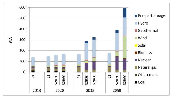
Figure 81. Electricity generating capacity for Canada
