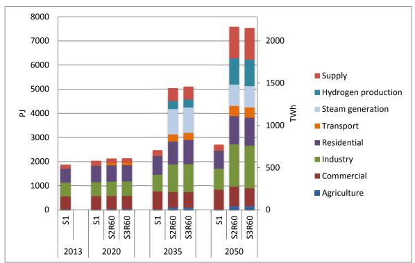
Figure 88. Electricity consumption - S1, S2R60 & S3R60
