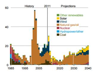
Figure 112. Additions to electricity generating capacity, 1985-2040 (GW)
